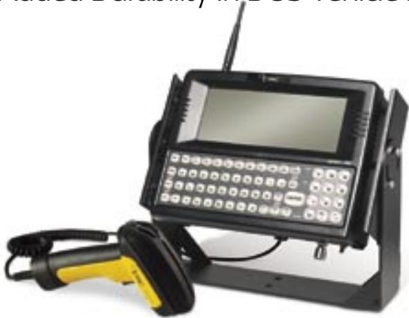
The Falcon® 625 is designed to excel in the harshest environments. Equipped with a IP66 sealed enclosure, the 625 is highly resistant to extreme temperature, vibration and impact.
