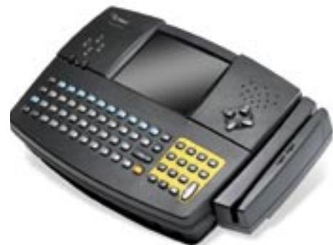
The Falcon® 515 fixed station computer features a 15 line x 40 character color or monochrome display, an IP54 enclosure rating, 2PC card slots, 2 serial ports, and 2 input ports for a variety of devices such as Power-Scan™ handheld scanners or mag stripe readers. The Falcon® 515 also features enhanced, relay-protected digital I/O ports to control devices such as warehouse carousels, light tables, locking mechanisms, and more for a maximum of automation flexibility.
